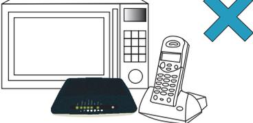
Do not place your router next to metallic objects, microwaves, cordless phones or RF transmission devices as these send out radio signals which can interfere with your router,
