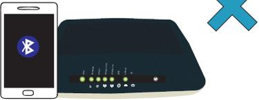
Bluetooth equipped devices like mobile phones send out radio signals. which can interfere with your router. Try turning these off one at a time to see if it make a difference.
